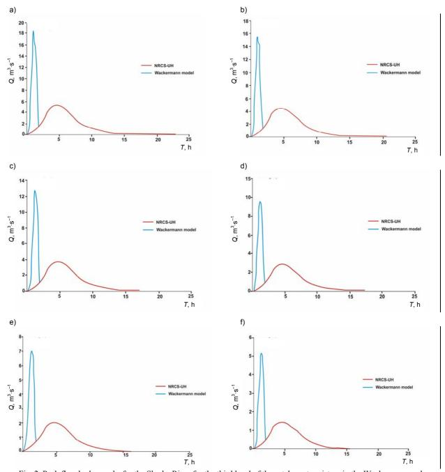
Fig. 2. Peak flow hydrographs for the Słonka River for the third level of the catchment moisture in the Wackermann and NRCS-UH model and the probability of a) 0.5%, b) 1%, c) 2%, d) 5%, e) 10%, f) 20%; source: own study
