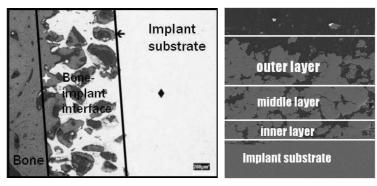
Fig. 2. (left) The cross section of the bone-implant interface created by adaptive ingrowth of bone tissue into pore space of the porous coating and (right) the cross section of a typical porous coating with symbolically distinguished layers: outer layer, middle layer and inner layer of which the outer layer is the subject of our research.
