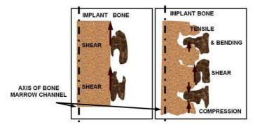
Fig. 3. Smooth vs. porous implant-bone interface.
