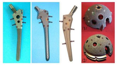
Fig. 4. The examined components of total hip arthroplasty endoprostheses: (from left to right) Johnson & Johnson Orthopaedics stem (Great Britain), Aesculap<sup>®</sup> stem, Biomet Merck Ltd. stem (Great Britain) and two acetabular Biomet Merck Ltd. cups /1/ & /2/ (Great Britain).
