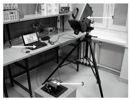
Fig. 6. Scattering measurement system: 1 -spectroradiometer CS-2000A, 2 -computer with dedicated software, 3 -measurement setup.
