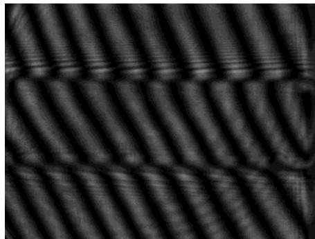
Fig. 10. Fringe pattern obtained during measurement of a 300mm long gauge block.
