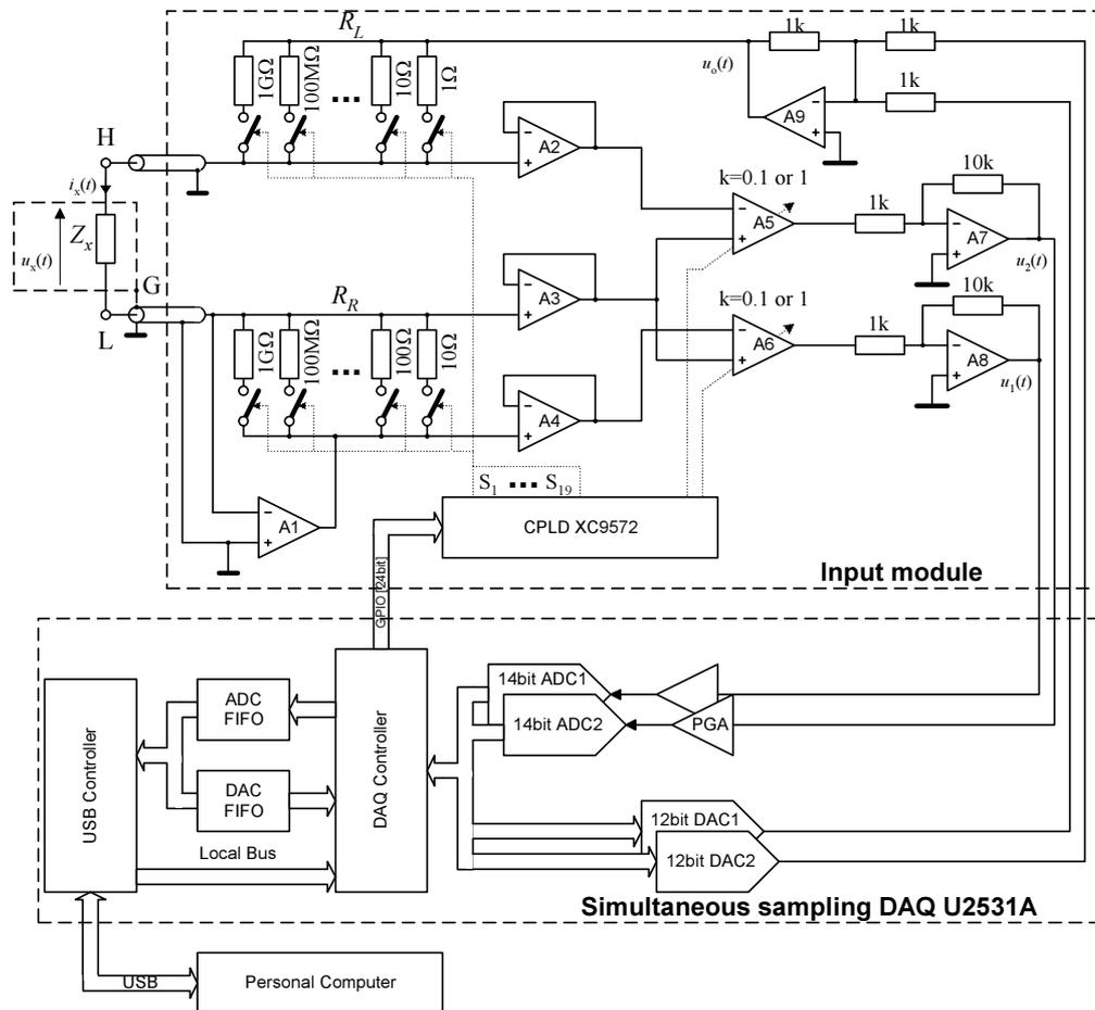
Fig. 5. Block diagram of the system for impedance spectrum measurement using sinc signal excitation.
