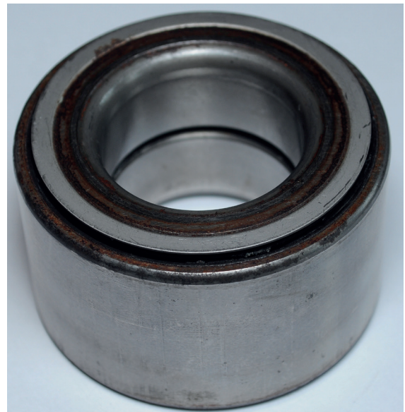
Fig. 4. Bearing VKBA 6831 from wheel of Toyota Avensis
