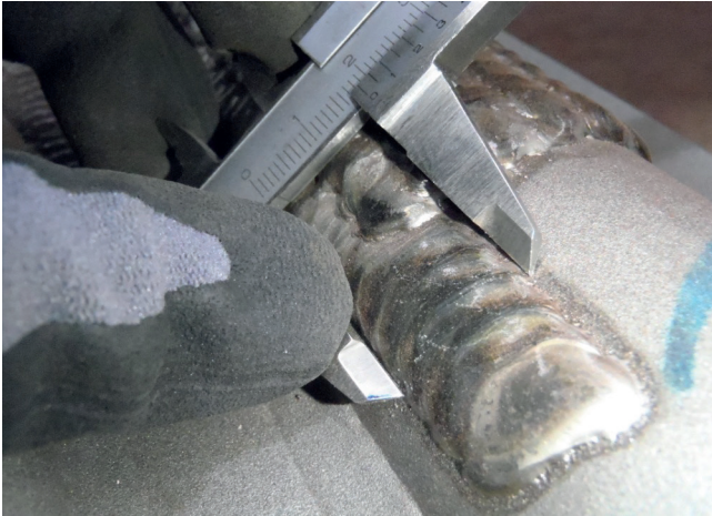
Fig. 5. Bead made by the CMT method. Width of the bead is about 18 mm, and its thickness is 1,8 mm
