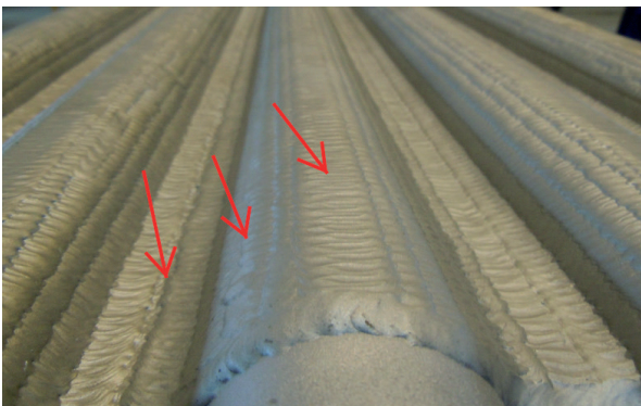
Fig. 14. Places of examining a content of iron on the surface of the surfacing weld
