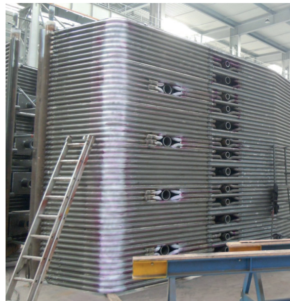
Fig. 15. Surfaced by welding and bent part of sheet pile wall of the boiler after PT
