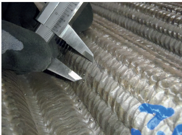
Fig. 6. Measurement of the beads' thickness
