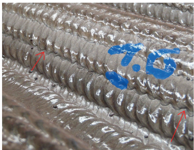
Fig. 8. Systematic irregularities on the beads' boundaries – "fastener effect"
