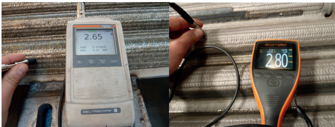
Fig. 9. Devices used to measure the thickness of the Inconel 625 surfacing weld
