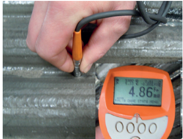
Fig. 11. Measurement of the thickness of the Inconel 625 surfacing weld on the flat bar
