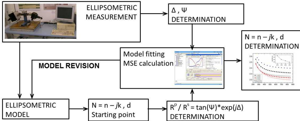
Fig. 1. The scheme of the ellipsometric measurement algorithm.
