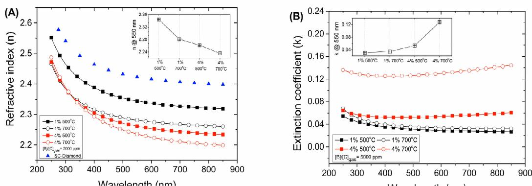
Fig. 3. Wavelength-dependent variability of (A) the refractive index  $n$  and (B) the extinction coefficient  $k$  in boron-doped diamond films deposited under various conditions related to the methane admixture and the substrate temperature. For comparative purposes, the refractive index measurements for a single-crystal diamond are shown ( $\blacktriangle$ -SCD) [41]. Insets: the variability of  $n$  and  $k$  measured at 550 nm.
