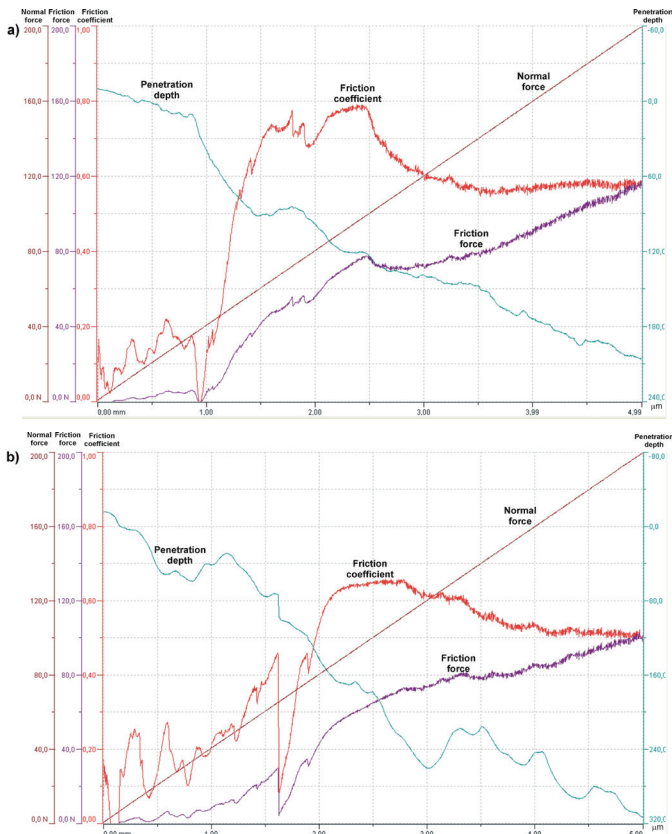
Fig. 11. Graph of data obtained from the scratch test for a preset force of 1 ÷ 200 N: (a) inner surface, (b) outer surface
