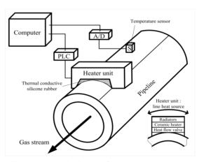
Fig. 1. A schematic diagram of the measurement system.
