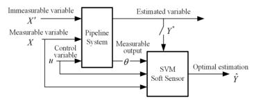
Fig. 2. The basic structure of SVM soft-sensor.
