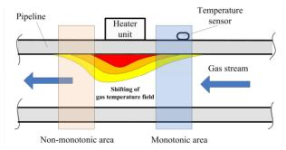
Fig. 3. A schematic diagram of sensor installation.
