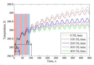
Fig. 5. The temperature time series at different flow rates for the multiple pulse mode.
