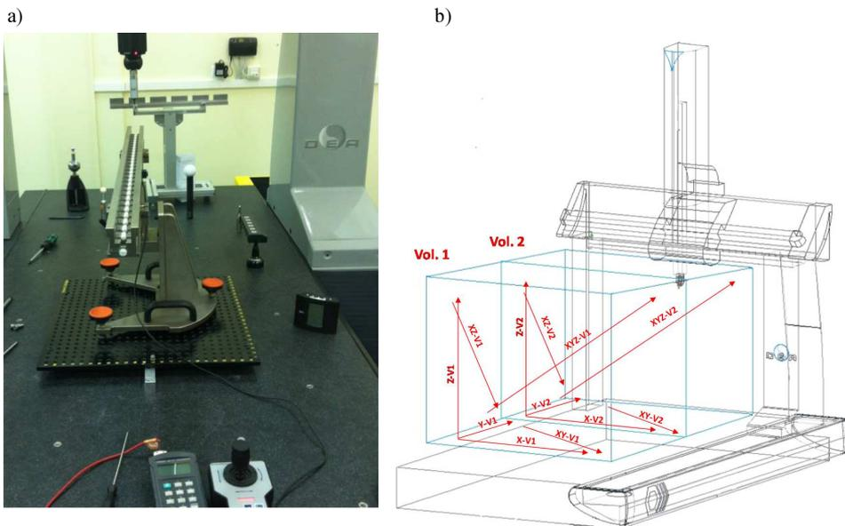
Fig. 2. a) The CMM during preliminary calibration (with KOBA® gauge) before the beginning of the experiment; b) Some volumes and orientations considered for posterior interim tests.
