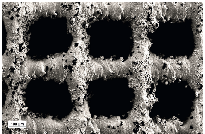
Fig. 6. Scaffold made of Ti6Al4V alloy in SLS/SLM process after etching in water solution with hydrofluoric acid for 8 minutes, SEM, magnification of 200x
