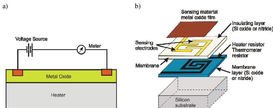
Fig. 5. a) The operation concept of a typical semiconductor gas sensor; b) an example of its construction.
