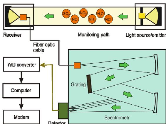
Fig. 14. A schematic of the DOAS sensor [49].
