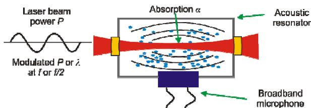
Fig. 16. The concept of photoacoustic spectroscopy [59].
