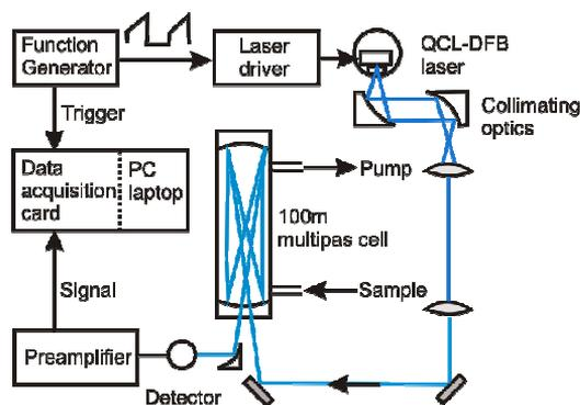
Fig. 13. A schematic of the TDLAS-MUPASS sensor [44].
