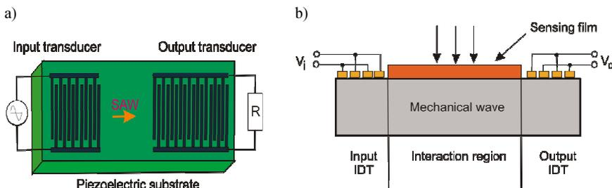
Fig. 6. a) The operation concept of a typical SAW gas sensor; b) its structure.
