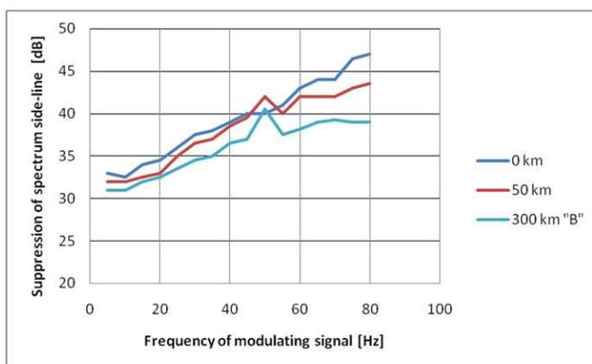
Fig. 7. The low-frequency noise suppression in TFTS-2 links.
