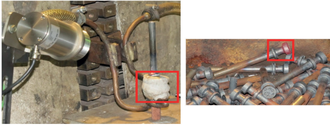
Fig. 7. Local induction heating of a forging
