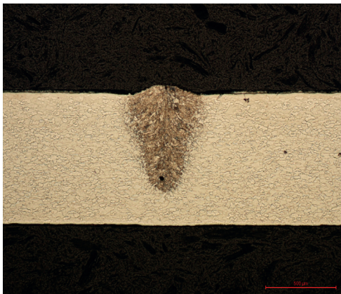
Fig. 1. Microstructure of the 0.8 mm thick electro-galvanized steel sheet DC04, 3% Nital etched, Table 1
