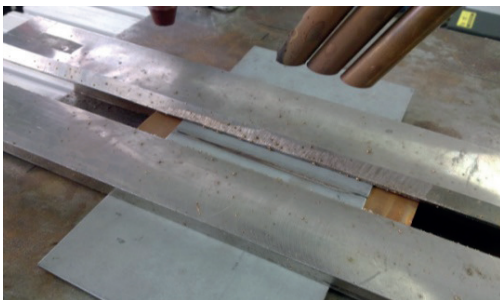
Fig. 2. A view of the clamping device applied for laser welding of 0.8 mm thick electro-galvanized steel sheet DC04
