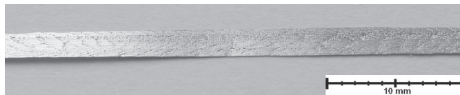
Fig. 2. Image of the AlSi11,6Mm4 alloy ribbon surface cast at a speed of 15 m/s, wheel-facing side
