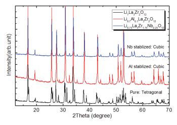
Fig. 1. XRD of the tetragonal, Al and Nb stabilized cubic  $\rm Li_7La_3Zr_2O_{12}$  compounds
