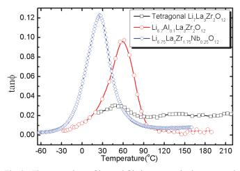
Fig. 2. The comparison of internal friction spectra in the tetragonal and Al, Nb stabilized cubic  $Li_7La_3Zr_2O_{12}$  compounds; the excitation frequency, f=1 Hz
