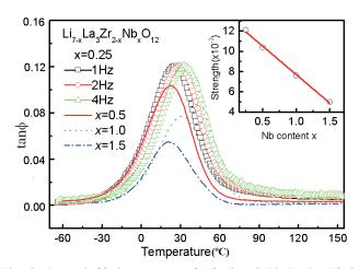
Fig. 3. Internal friction spectra of Nb doped  $Li_{7-x}La_3Zr_{2-x}Nb_xO_{12}$  samples. Inset: the peak height as a function of Nb content *x*
