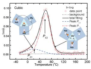
Fig. 4. Fitting results of the  $P_C$  peak and diffusion model of lithium ions: 496h $\leftrightarrow$ 96h for peak  $P_{C1}$  and 96h $\leftrightarrow$ 24d for the  $P_{C2}$  peak
