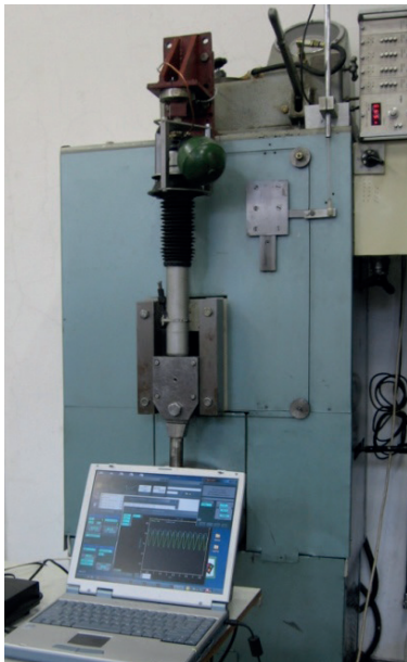
Fig. 5. Indicator-type testing station for determination of dynamic characteristics of a hydropneumatic strut
