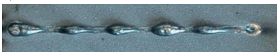
Fig. 10. A view of the humped root of bead-on-plate welds, as a result of key hole instability, produced at 3300 W and welding speed: a) 1300 mm/min (152.8 J/mm), b) 1750 mm/min (113 J/mm)
