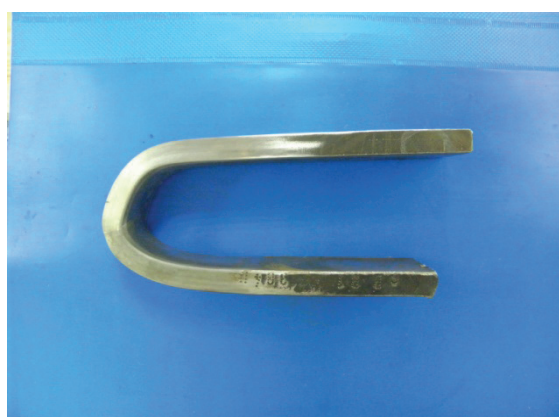
Fig. 6. A phenomena of non-axial deformation of bent samples
