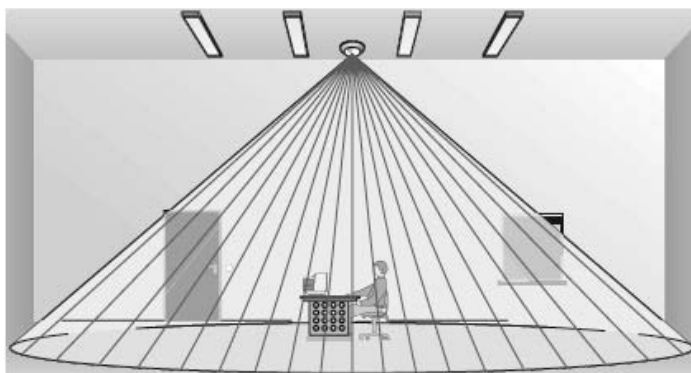
Fig. 7. Use of movement sensor detecting human occupancy in the room for lighting control [1]
