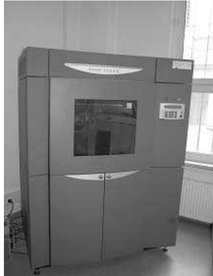
Fig. 1. FDM Titan device made by Stratasys
