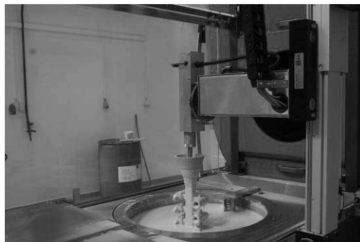
Fig. 3. Application of ceramic coating
