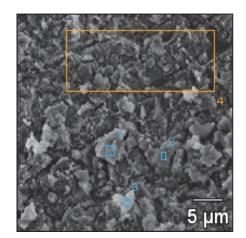
Fig. 2 Structure of catalytic converter sample with marked selected areas for X-ray energy spectra
