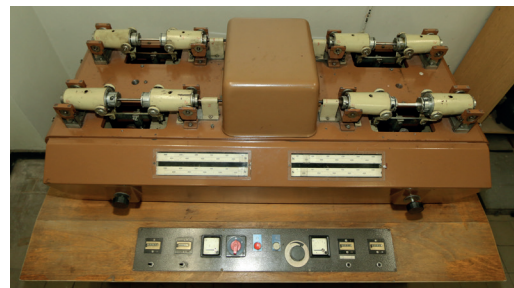
Fig. 1. Machine for high-cycle fatigue testing under conditions of rotary bending
