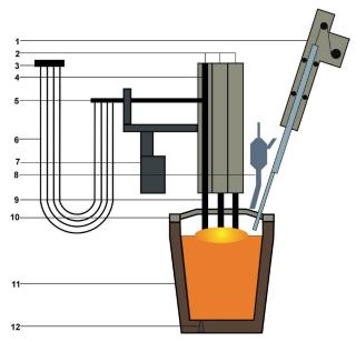
Fig. 1. Scheme of the ladle furncae (LF) station [1]. 1 - ladle, 2 – automatic temperature measuring and metal & slag sampling instrument, 3 – analyzer, 4 – LF operator's computer, 5 – Argon supply, 6 – ferroalloy reservoirs, 7 – automatic scales, 8 – charge chute
