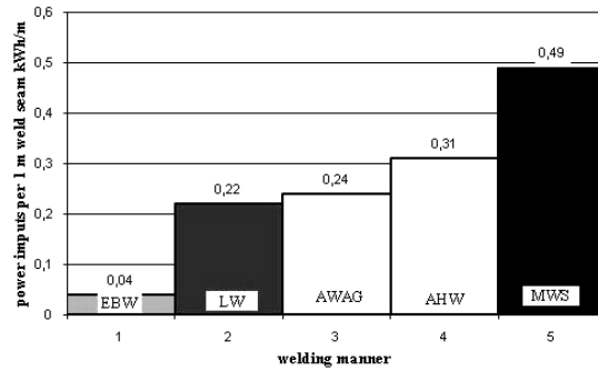
Fig. 3. Cost sharing of electrical energy per 1 m of stitch of the connection C4 for various ways of the welding: EBW – electron-beam welding, LW – laser welding, AWAG – automatic arc welding in active gases, AHW – automatic hidden arc welding, MWS – manual arc welding
