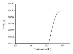
Fig. 2.  $Al_2O_3$  content during S235 steel solidification at a cooling rate of 50 K/min
