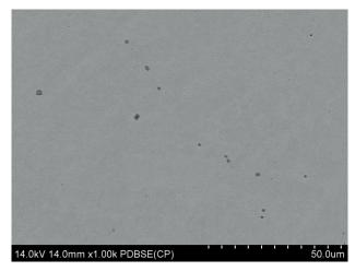
Fig. 8. The non-metallic precipitates distribution in the cast steel ingot (SEM)
