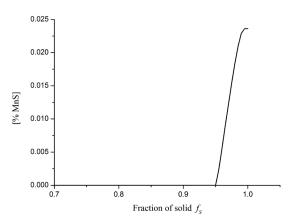
Fig. 6. MnS content during S235 steel solidification at a cooling rate of 50 K/min
