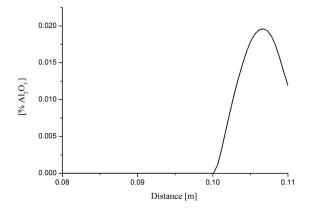
Fig. 3.  $Al_2O_3$  content during S235 steel solidification at a cooling rate of 50 K/min (distance from the wall to the center of the ingot 0.11 m)
