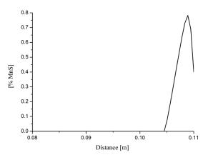
Fig.7. MnS content during S235 steel solidification at a cooling rate of 50 K/min (distance from the wall to the center of the ingot 0.11 m)
