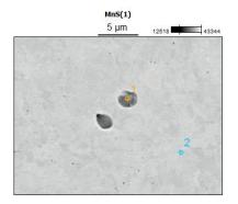
Fig. 11. Morphology and distribution of the non-metallic precipitates in the cast steel ingot
