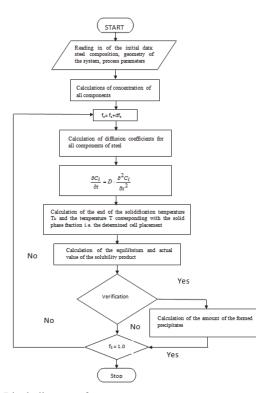
Fig. 1. Block diagram of computer program
