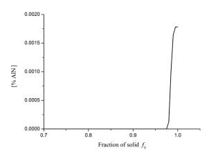
Fig. 4. AlN content during S235 steel solidification at a cooling rate of 50 K/min
