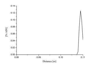
Fig. 5. AlN content during S235 steel solidification at a cooling rate of 50 K/min (distance from the wall to the center of the ingot 0.11 m)
