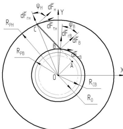
Fig. 1. The scheme of constructing of stator slot
