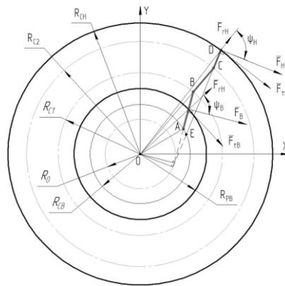
Fig. 2. Scheme of the combined slot of stator
