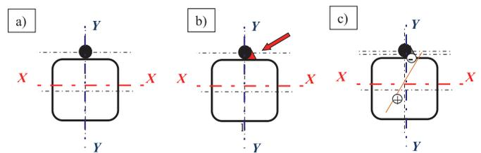
Fig. 1. A scheme of a cross-section of a metal wire mesh with a frame in the place of joining: a) with a distribution of axes of inertia on the section, b) with a distribution of axes of inertia on the section, and the weld causing stresses, c) with a distribution of axes of inertia on the section, and the stresses which cause deformations of an element
