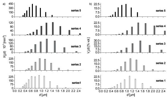
Fig. 2. The grain size distribution a) the dependence of the  $N_A$  grain number of a given size on the unit area on the d grain size (the statistical distribution), b) the dependence of the  $V_{\nu}$  grain volume of a given size on the d grain size (the geometrical distribution)
