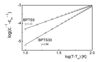
Fig. 4. The dependences of  $\log(\varepsilon^{-1} - \varepsilon_m^{-1})$  vs.  $\log(T - T_m)$  at 1 MHz for BPTS5 and BPTS30 samples
