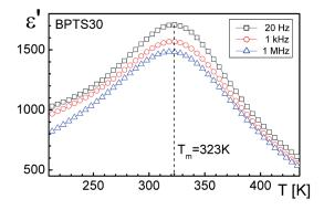
Fig. 3. Temperature dependence of the real part of dielectric permittivity  $\epsilon^\prime$  for BPTS30 at the frequency of 20 Hz, 1 kHz and 1 MHz
