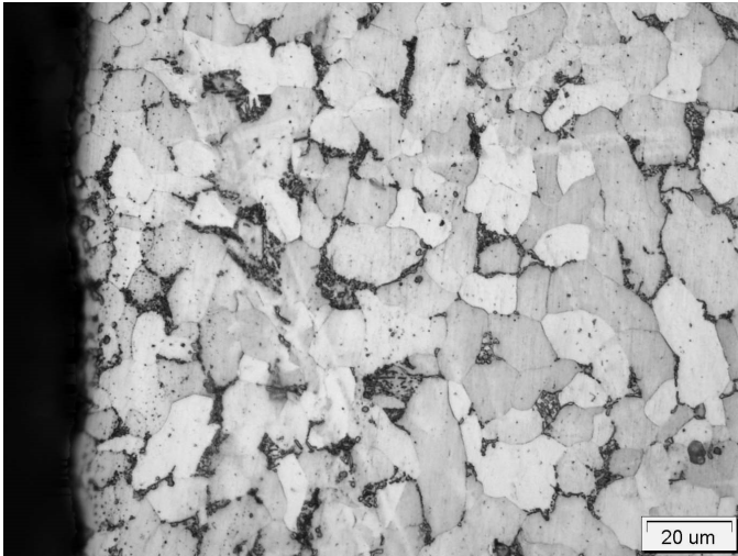
Fig. 3. Ferrite grains with granular cementite in the plate of element 4. Surface area – Nital etching
