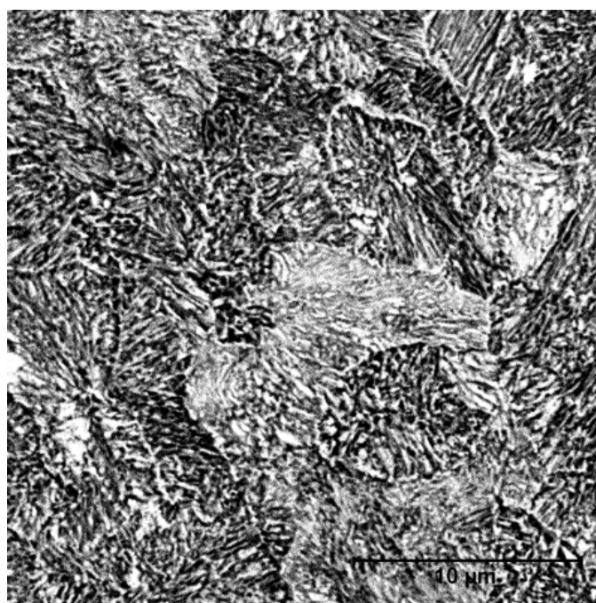
Fig. 2. Magnified area of structure shown in Fig. 1, visible hard, and hardly etching cementite lamellae protrudes over the soft ferrite. SEM
