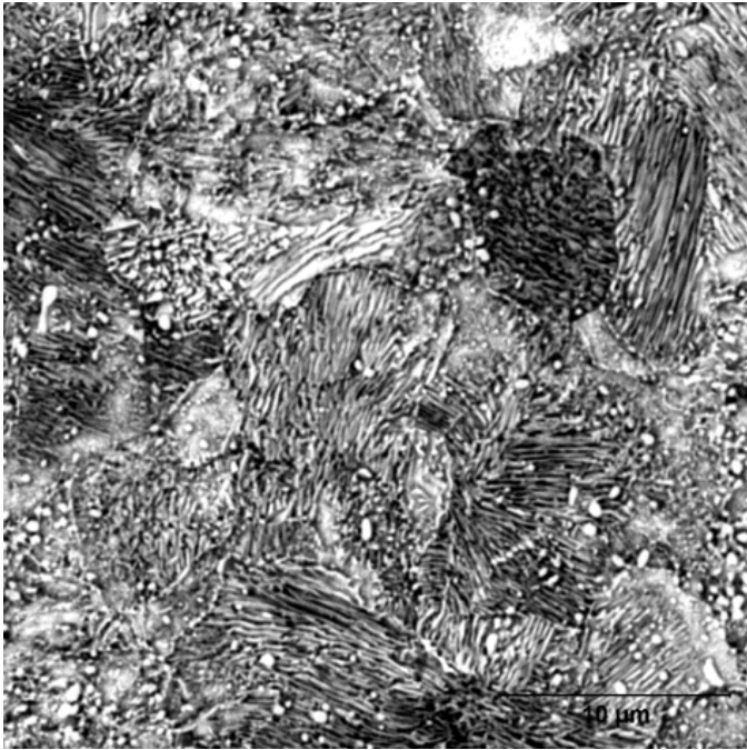
Fig. 6. Microstructure of material after modification at 500°C, visible numerous spherical disengagement of cementite in the ferritic matrix. SEM
