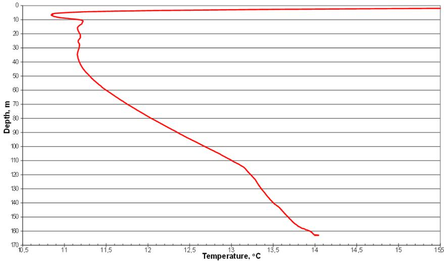
Fig. 4. Measured temperature profile of borehole heat exchanger P-2 (double u-tube) in terms of thermal stability
