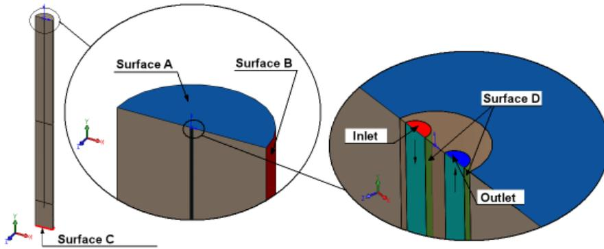
Fig. 2. Description of surface for initial and boundary conditions
