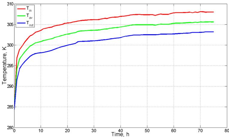
Fig. 13. The temperature changes on the supply and return of borehole heat exchanger
