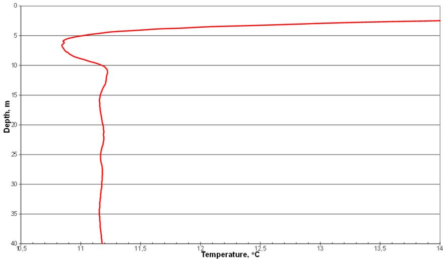
Fig. 5. Measured temperature profile of borehole heat exchanger P-2 in interval 0-40 m
