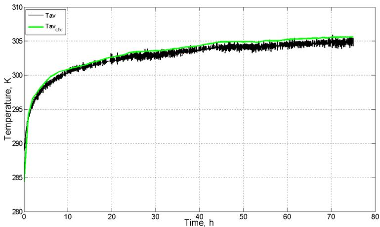
Fig. 14. Average heat carrier temperature changes for measurement and simulation data
