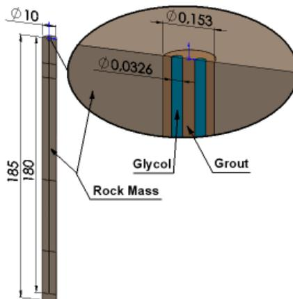
Fig. 1. Object of research – model of heat exchanger, a single U-tube
