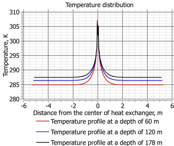
Fig. 10. Temperature changes at depths of 60 m, 120 m, 178 m
