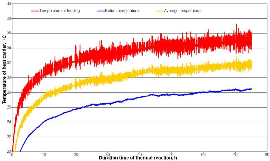
Fig. 8. Results of temperature measurements during TRT of borehole heat exchanger P-1 (single U-tube)
