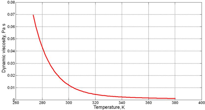
Fig. 3. Dynamic viscosity of 33% propylene glycol, Pa · s (Chem Group, 2011)
