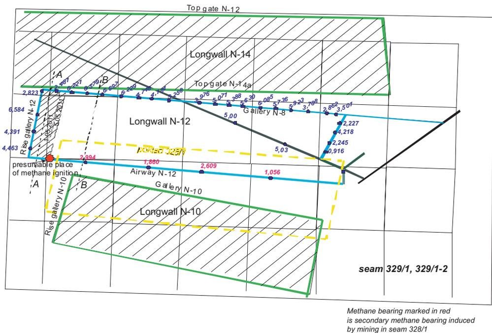
Fig. 2. Planned mining of seam 329/1, 329/1-2 with longwall N-12
