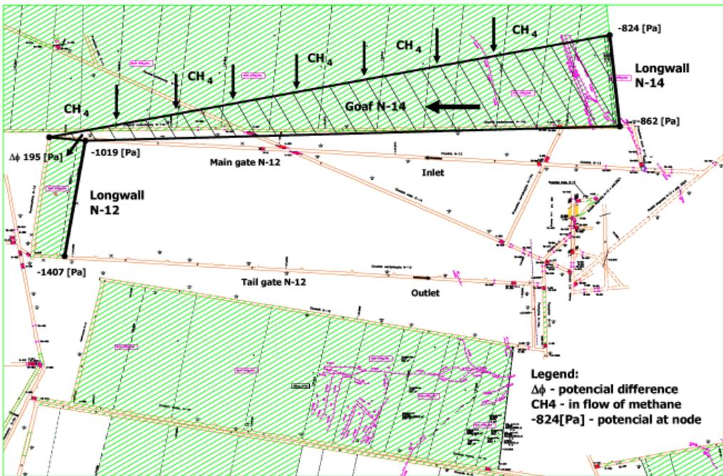
Fig. 6. Shaping of the tendency of goaf gases migration including methane in goaf between longwalls N-14 and N-12 goaf in seam 329/1, 3129/1-2
