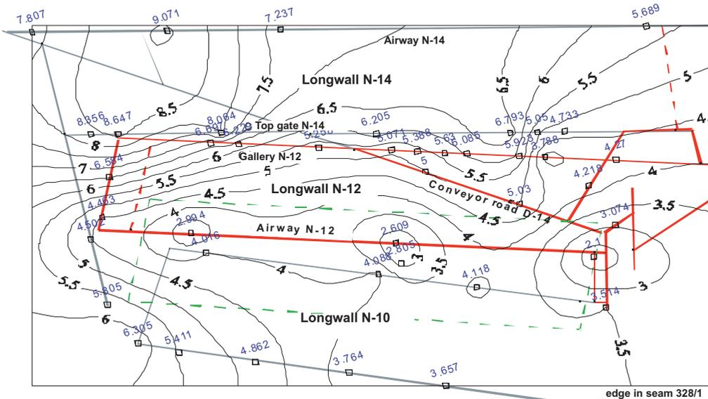
Fig. 1. Map of the isoline of methane-bearing capacity on the panel length of longwall N-12 in seam 329/1, 329/1-2 in hard coal mine "Krupiński"
