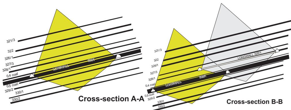
Fig. 3. Zones of destressing with longwalls in seams 329/1, 329/1-2 and 328/1, not de-stressed part (cross-section A-A) and de-stressed part (cross-section B-B) from Figure 2
