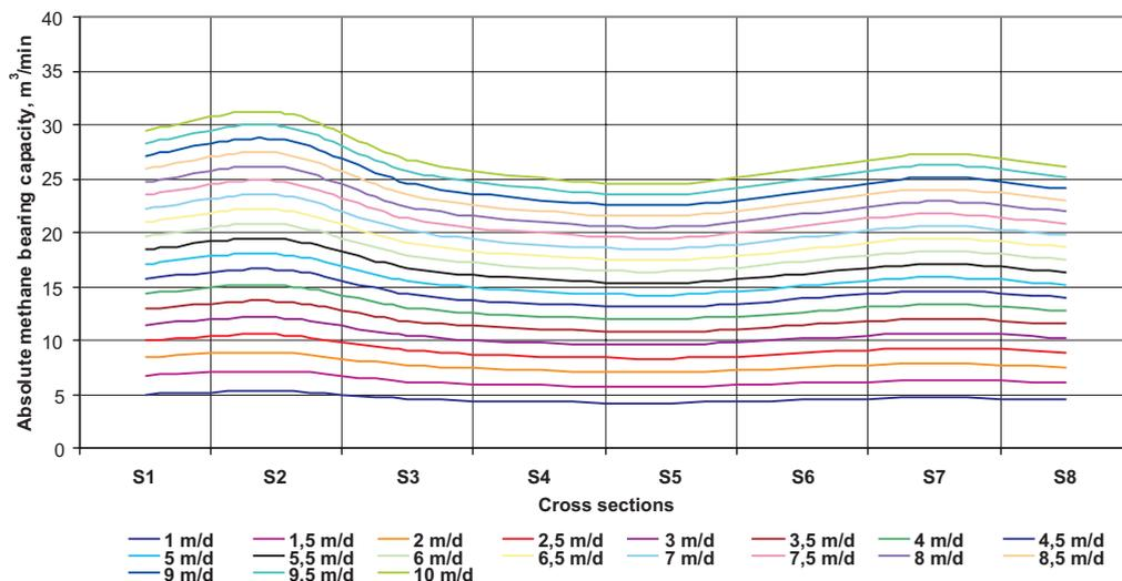
Fig. 4. Forecasts of methane emissions on designed panel length of longwall N-12 in the scope of advances 1-10 m/d
