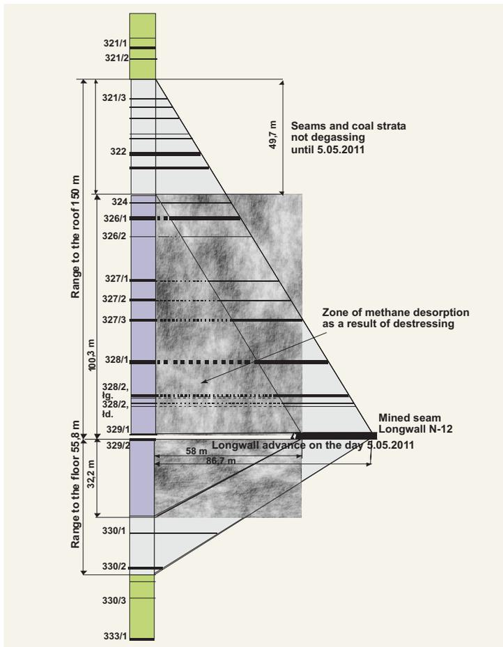
Fig. 5. Zone of destressing and degasification of undermined and overmined coal-beds of longwall N-12 in seam 329/1, 329/1-2 after reaching advance of 58 m on 5.05.2011
