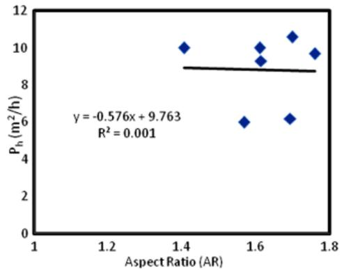
Fig. 6. Relation between production rate and Aspect Ratio
