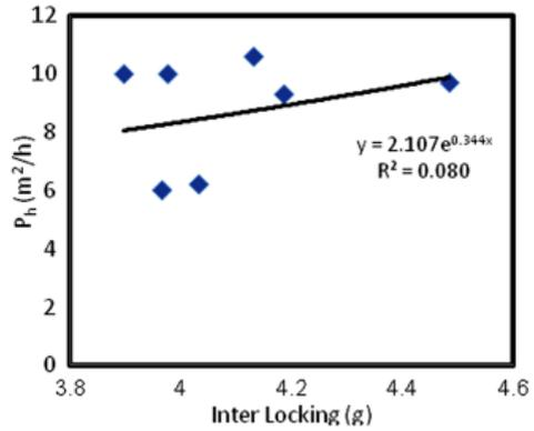
Fig. 10. Relation between production rate and texture coefficient
