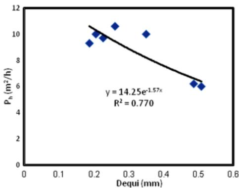
Fig. 7. Relation between production rate and Diameter equivalent
