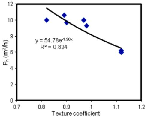
Fig. 3. Relation between production rate and texture coefficient
