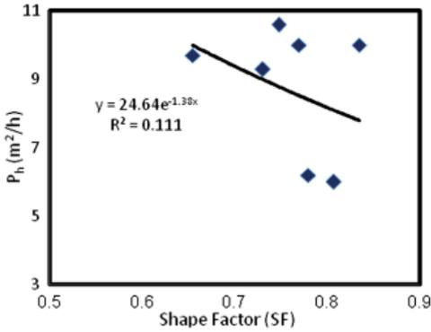
Fig. 9. Relation between production rate and texture coefficient
