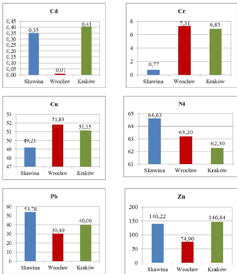
Fig. 3. Total contents of selected heavy metals in mg · kg<sup>-1</sup> in ashes from Combined Heat and Power Plants Skawina and Kraków and in ash slags from EC Wrocław
