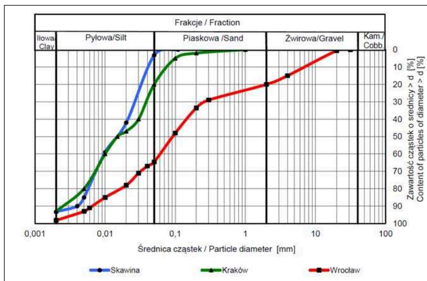
Fig. 2. Grain size distribution curves of the tested wastes
