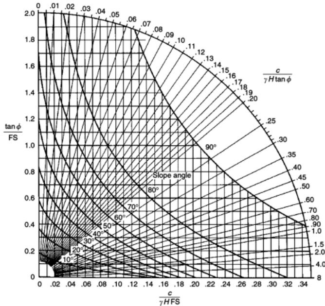
Fig. 6. Circular failure chart [8]
