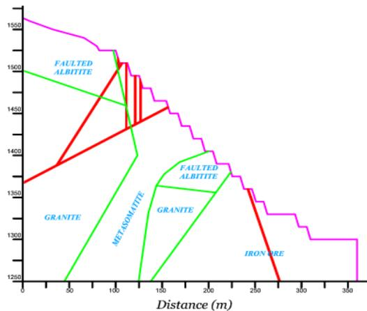
Fig. 8. Geological cross-section of Chadormalu iron open pit mine southern wall
