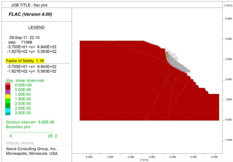
Fig. 4. Calculated safety factor by FLAC software
