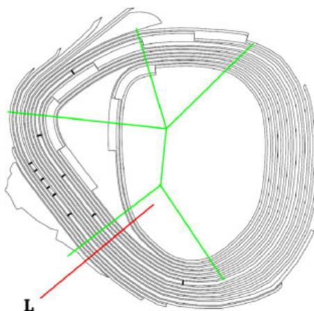
Fig. 2. Geotechnical sections in Chadormalu iron open pit mine and studied cross-section in southern wall (Kani Kavan, 2008)
