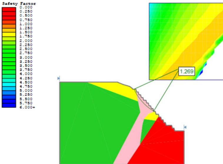
Fig. 5. Safety factor calculated by SLIDE software
