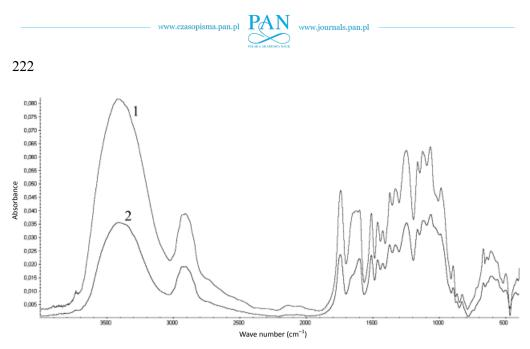
Fig. 5. The comparison of the IR spectra obtained for walnut shells samples before (1) and after the process of  $Pb^{2+}$  sorption (2)
