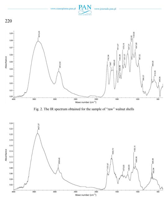
Fig. 3. The IR spectrum obtained for the sample of "raw" sunflower hulls
