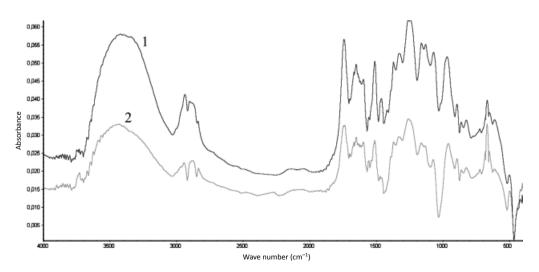
Fig. 4. The comparison of the IR spectra obtained for plum stones samples before (1) and after the process of Pb<sup>2+</sup> sorption (2)
