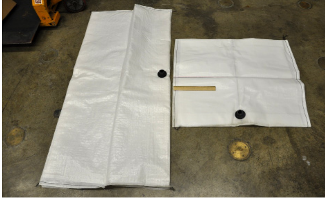
Fig. 2. Photograph of two typical grout bags
