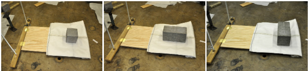
Fig. 4. Concrete block orientations. Half, full orientation A, full orientation B
