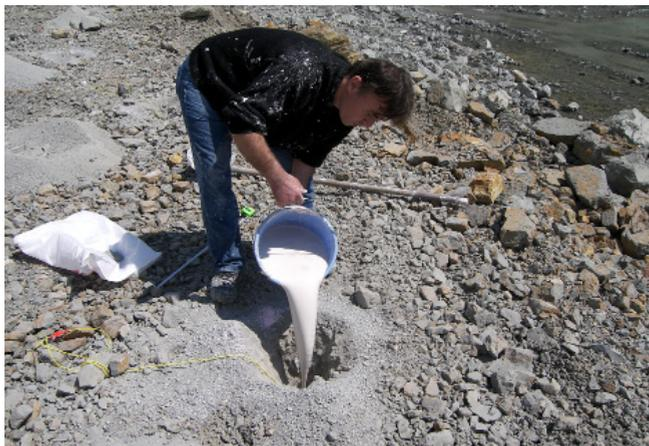
Fig. 1. Application of plaster paste to hole collar
