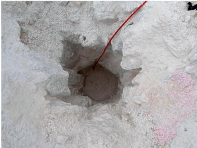
Fig. 3. Cracked hole collar and hardened plaster
