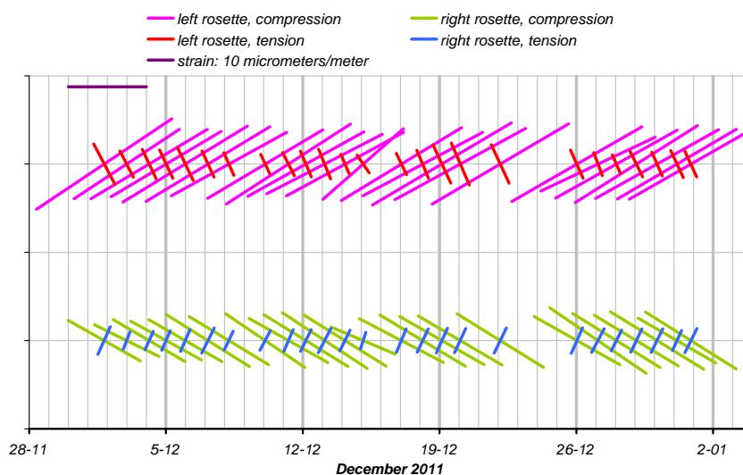
Fig. 10. The main strains of the constituent slabs making up the main slab, in the spots where the rosettes were located, for each case of stationing an aircraft in December 2011
