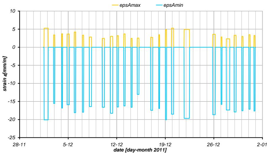
Fig. 7. The left rosette. The values of the main strains: the maximum ( $\text{epsAmax}$ ) and the minimum ( $\text{epsAmin}$ ) ones, caused by the aircraft load to the main slab. December 2011
