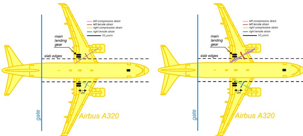
Fig. 8. A graphical interpretation of the measurement results: the values and the main strains for a particular recorded case of stationing an aircraft in the hangar
