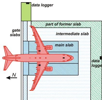
Fig. 3. The plan of the hangar slab after modernization – the eastern part
