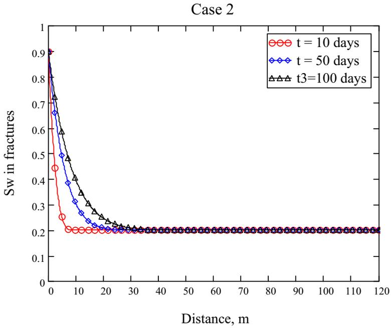
Fig. 2. Water saturation in fractures, Case 2,  $A = 4.129E-3 s^{-0.5}$
