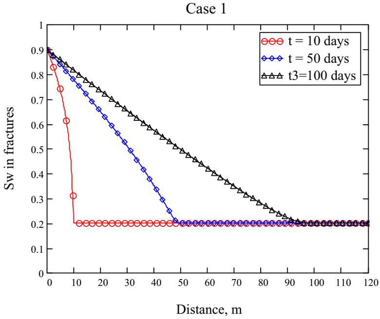
Fig. 1. Water saturation in fractures, Case 1,  $A = 4.129E-4 s^{-0.5}$
