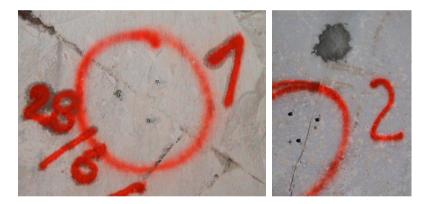
Fig. 10. Visual (cement seal) and manual (three screw system) measurement of the displacements of open dikes within safety pillars
