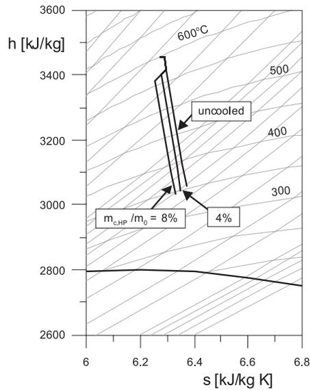
Figure 8. High pressure expansion with and without cooling.
