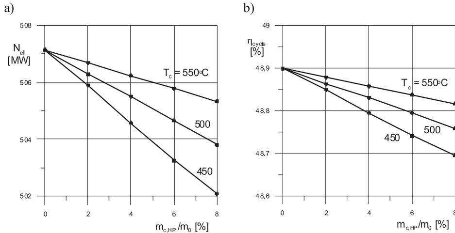
Figure 7. Power output and power generation efficiency for various cooling conditions in the HP turbine part and live steam temperature  $600^\circ\text{C}$ .
