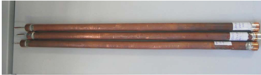
Figure 2. Water heat pipes with sintered capillary structure.
