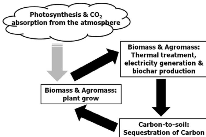
Figure 3. Enhanced biomass-to-energy cycle with biochar sequestration.
