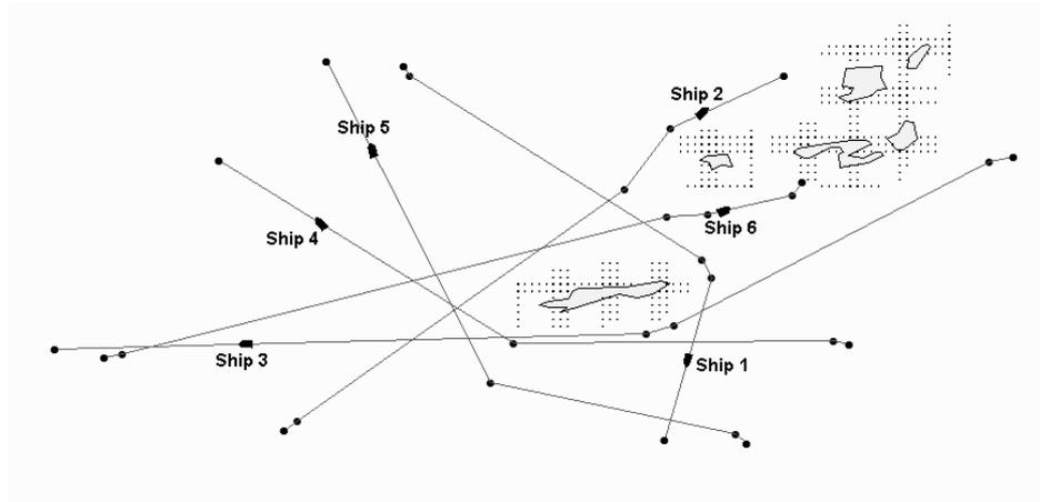
Fig. 12. Restricted water scenario – dotted areas depict shallow waters (positions after 80% of total simulation time)
