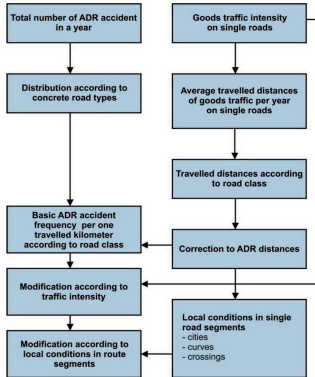
Fig. 2. Specific model of ADR accident frequency calculation on traffic roads
